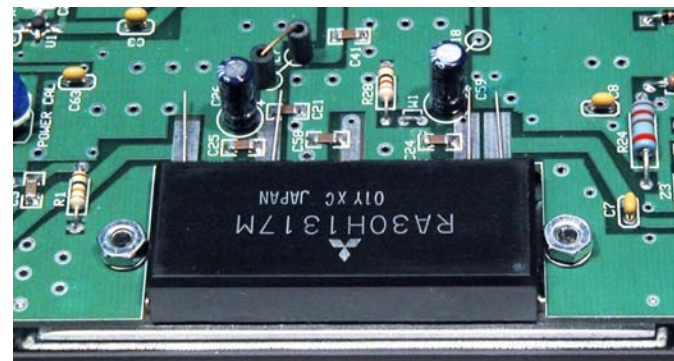
Figure 34. RF PCB attached to the RF Power Module Screws.
