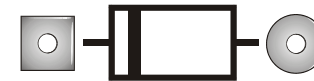
Figure 16. PCB Diode Orientation Guides. The cathode always goes to the square solder pad on the PCB.
